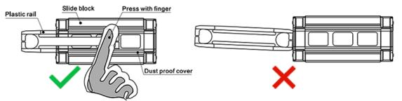
Press the dust-proof covers and insert plastic rail in alignment.
