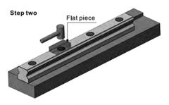
Place the flat piece on mounting hole, hit the piece vertically with a plastic hammer and fix the plug into counterbore.
